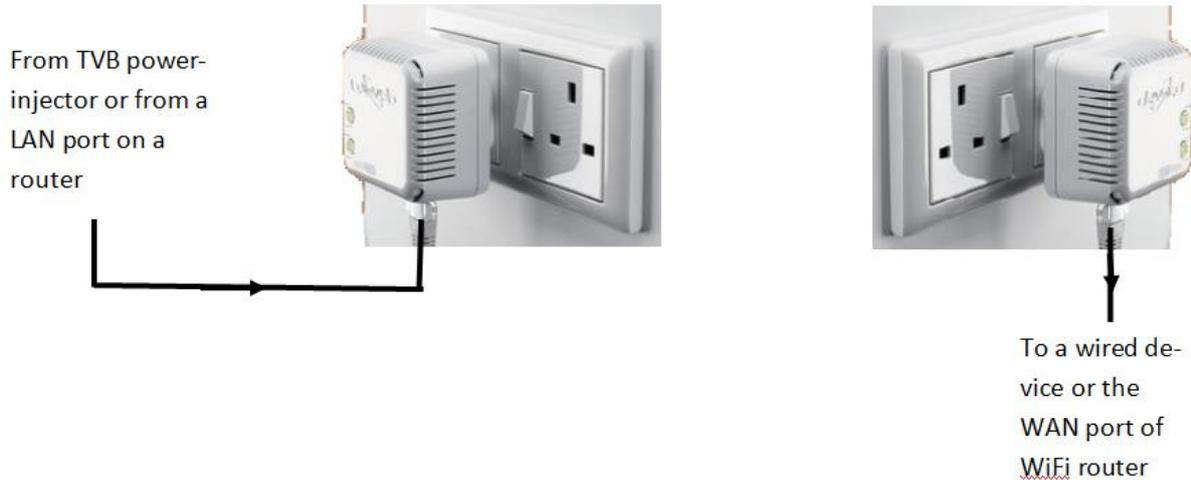
The secondary unit might have a Wi-Fi point access built-in and may have more than one Ethernet socket for connecting to wired devices.
