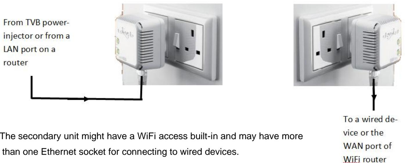
The secondary unit might have a WiFi access built-in and may have more than one Ethernet socket for connecting to wired devices.
