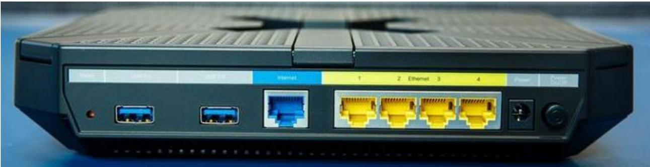
The LAN socket on your power injector (Radio broadband) or on the Optical Network termination (fibre broadband) should be connected to the WAN socket (sometimes labelled “Internet” and usually coloured differently from the other sockets).
