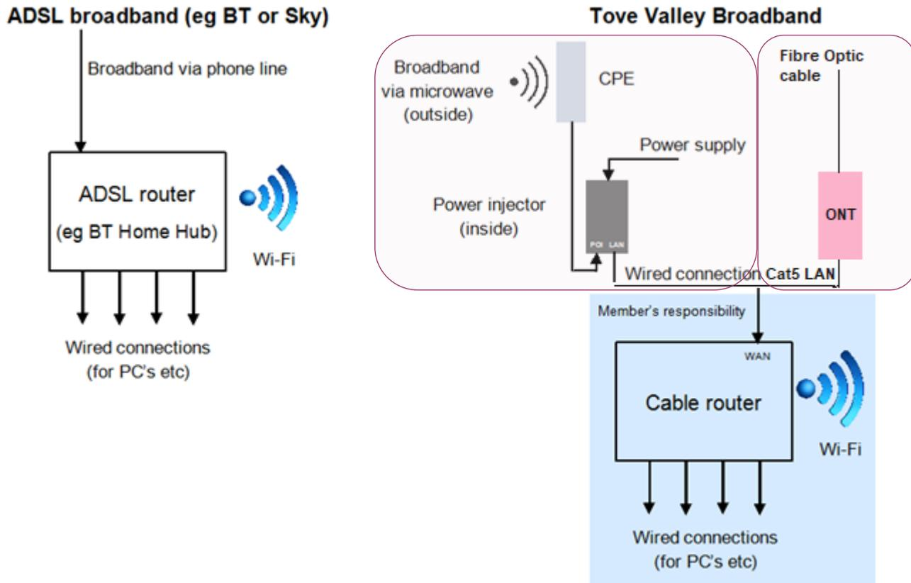
The TVB **radio** supply is via the Customer Premises Equipment (CPE) on the outside of your house and terminates in a single wired connection at the power injector inside your house. A **fibres-optic** cable supply is terminated in your house at an Optical Network Termination (ONT) which also provides a single wired connection. The service at this port is where the TVB responsibility ends.
