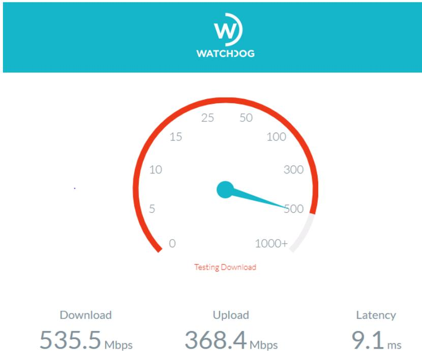
Latency is a measure of the speed of a message over the internet. For example, when gaming with others over the internet this is of paramount importance and (for gaming) should be less than 20ms. WiFi and radio can affect this.
